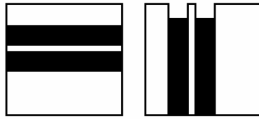
Figure 2: CD standard fabrication steps: (left) alternate layers of silicon (white) and silicon oxide (black) are deposited; (right) the wafer is then diced and rotated, and part of the oxide is etched, thus leaving a standing silicon line.
